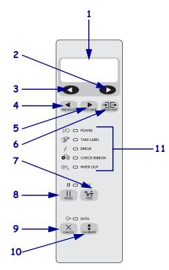
Figure 4 • Location of Control Panel Buttons and Lights
